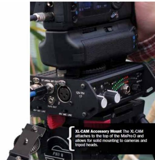
**XL-CAM Accessory Mount** The XL-CAM attaches to the top of the MixPre-D and allows for solid mounting to cameras and tripod heads.
