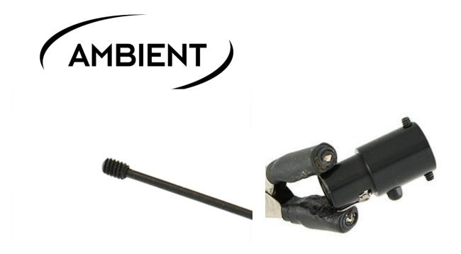
4. Remove the grub screws from the baggy and place on the hex wrench. Install the screws with just a few turns so they stop flush with the inside of the shell. We recommend getting a nice .9mm Hex driver like a Wiha brand driver if you build many cables as the tiny Hex wrenches seem to fail and strip quite easy.
