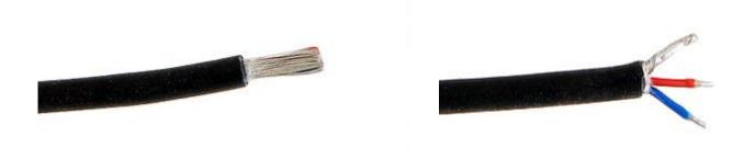
1. Remove approximately 6mm of the cable jacket. Fray and twist the shield tight and tin all leads. *Note: the ideal cable OD for LPS connectors is about 2.7mm to 3.0mm. Belden 1804A is about 2.9mm.*
